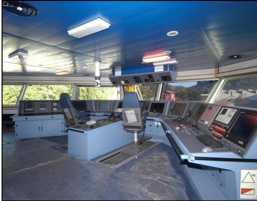
**Figure 6- Integrated Bridge System of Sagar Nidhi**
