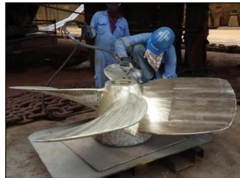
Figure 9- Hull & Propeller cleaning during dry-dock of Sagar Nidhi
