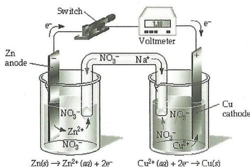
**Figure 2 – Electro-chemical Cell**
