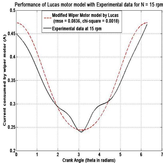
Figure 5: Performance of Modified Lucas Wiper Motor model with experimental data at 15 rpm.
