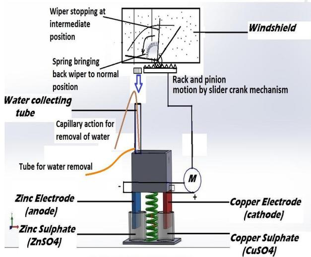
Figure 3: Schematic diagram of the electrochemical wiper mechanism
