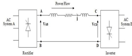
Figure 1 HVDC system model
