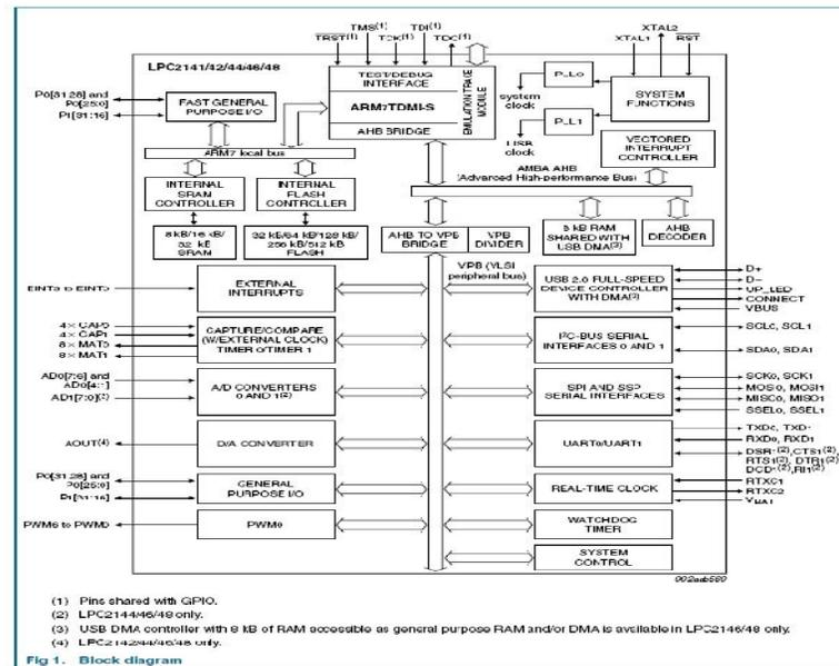
Fig. 2.3 BLOCK DIAGRAM OF ARM
