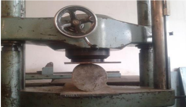
Figure 7 : Split tensile test
