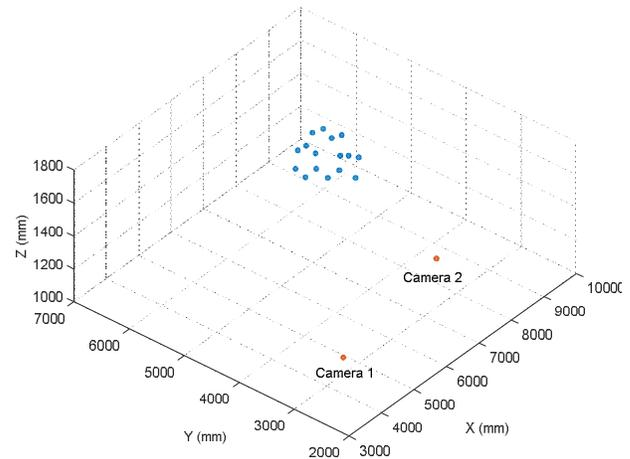
**Figure 5. Positions of the cameras and control points**
