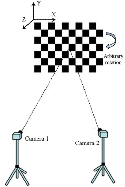
Figure 3. Checkerboard and two cameras for stereo calibration.
