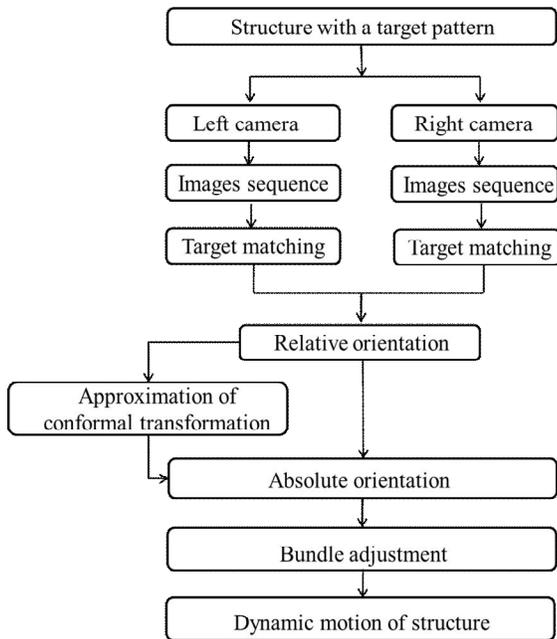
**Figure 1. Dynamic motion measurement procedure using two cameras.**
