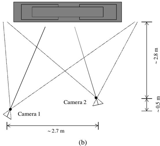
**Figure 4. Schematic overview of experimental setup; (a) configuration of measurement system and (b) position of cameras with respect to object.**
