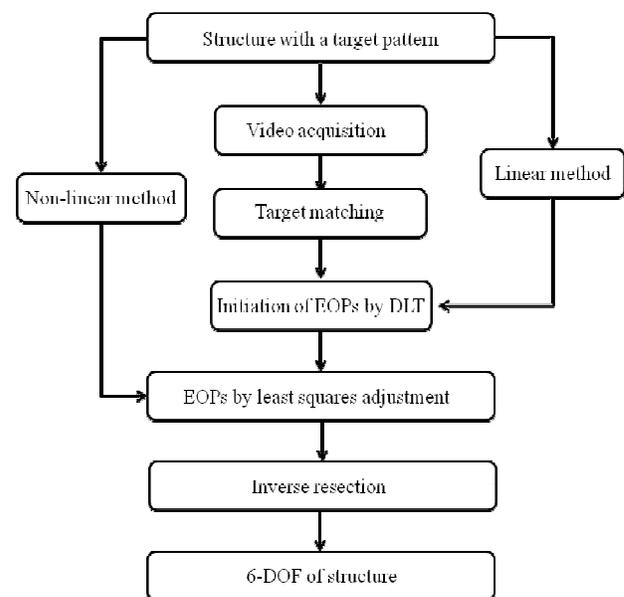
**Figure 2. Movement-measurement procedure using a single camera.**
