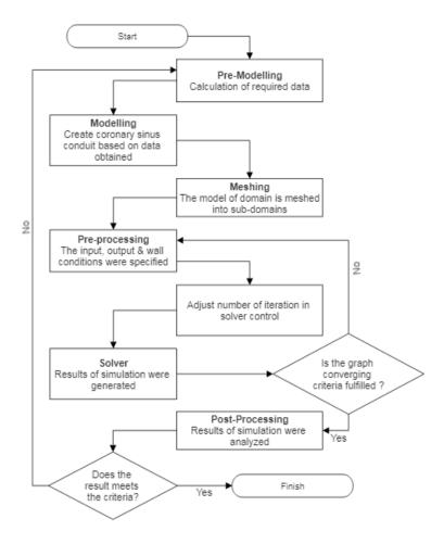
Figure 1: Flowchart of Finite Element Analysis
