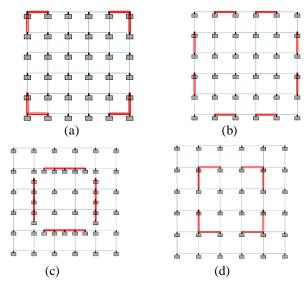
Figure 24: Shear Wall Positions
