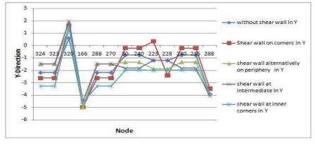
Figure 26: Comparison of node displacement in Y- direction
