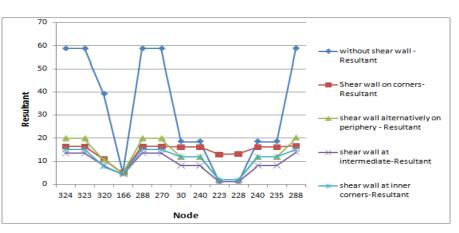
Figure 28: Comparison of Resultant node displacement.
