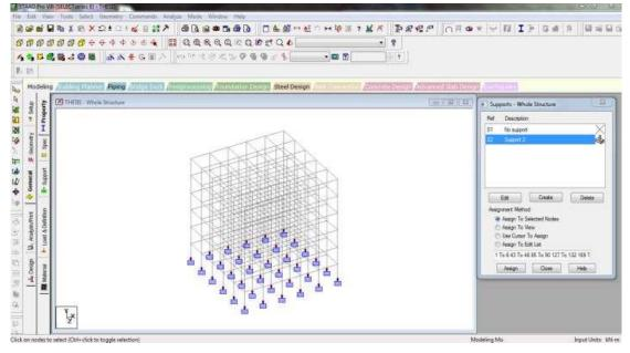
Figure 7: Structure with Fixed Supports
