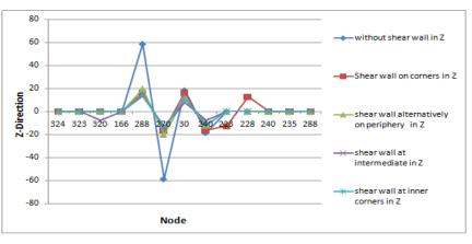
Figure 27: Comparison of node displacement in Z
