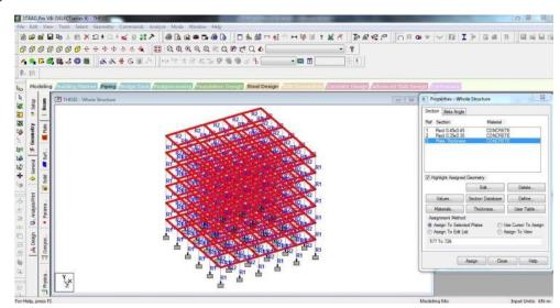
Figure 9: Slab properties
