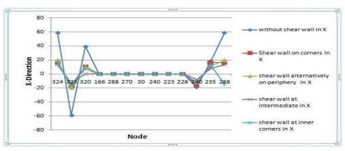
Figure 25: Comparison of node displacement in X- direction
