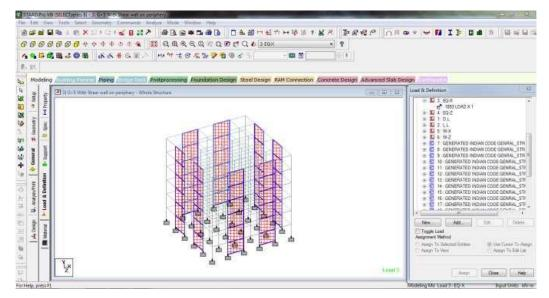
Figure 18: Model with shear wall alternatively on periphery
