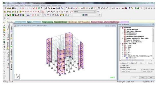
Figure 17: Model with shear wall on corners
