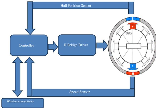
Figure 1: Block diagram for Embedded Ceiling Fan
