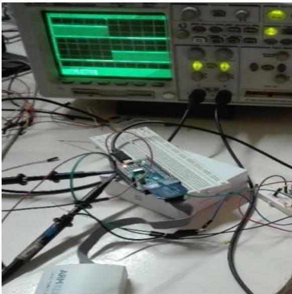
Figure 4: Test setup with ARM ULINKpro-D
