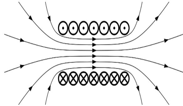
Figure 2: Magnetic field produced by a solenoid (coil of wire)
