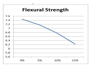
Figure 4: Flexural Strength for 0%, 5%, 10%, 15% replacement of Fine Aggregateby Crumb Rubber
