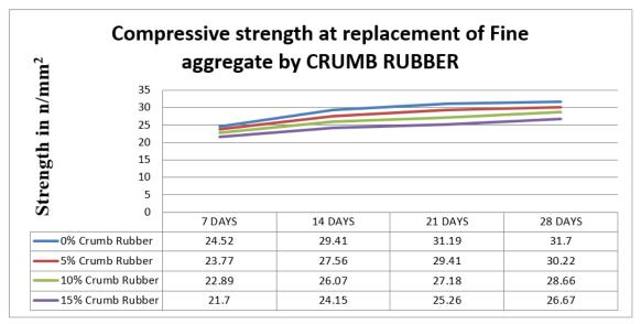
Figure 5: Compressive strength substitution of Fine Aggregate by Crumb Rubber after 7, 14, 21 & 28 days for M25
