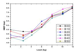
Fig. 10 Variation of IMEP with load
