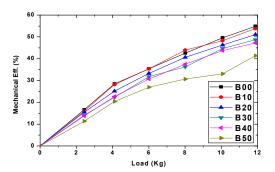
Fig .13 Mechanical Eff. vs. Load at CR 18
