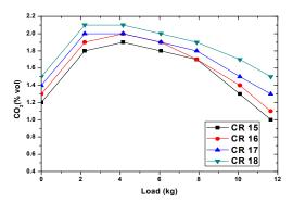
Fig .25 CO<sub>2</sub> variations with load at B50
