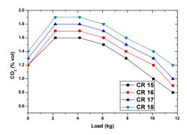
Fig .24 CO<sub>2</sub> variations with load at B10
