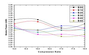
Fig.9 Variation of Brake Power with compression ratio at different blending
