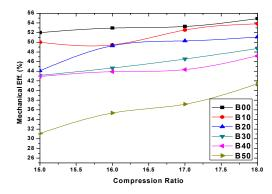
Fig. 14 Variation of Mechanical Efficiency with compression ratio at different blending
