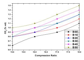
Fig.26 Variation of CO<sub>2</sub> with compression ratio for different blending
