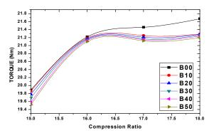
Fig.4 Variation of Torque with compression ratio at different blending
