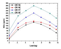
Fig .21 NOx variations with load at B10
