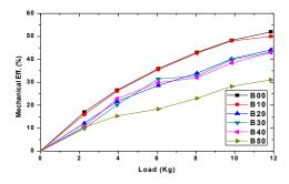
Fig .12 Mechanical Eff. vs. Load at CR 15
