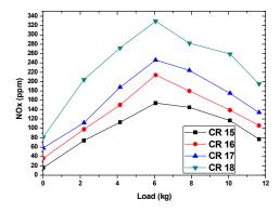
Fig .22 NOx variations with load at B50
