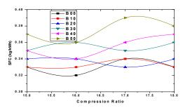
Fig.7 Variation of SFC with compression ratio at different blending
