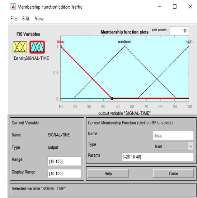
Figure 6: Membership Function of Output Variable Signal Time.
