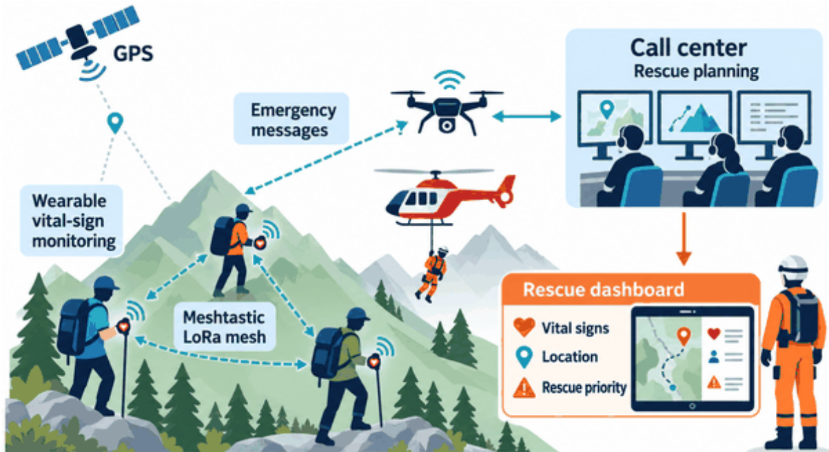
(a) Mountain rescue application scenario with wearable monitoring and LoRa mesh communication.
