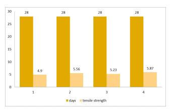
Figure 6: Split tensile strength in 28 day
