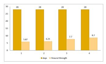
Figure 4: Flexural strength in 28 days
