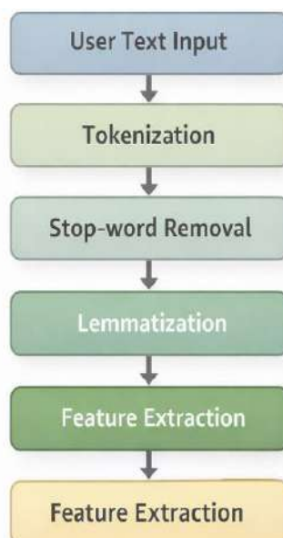
Figure 2: NLP Processing Pipeline
