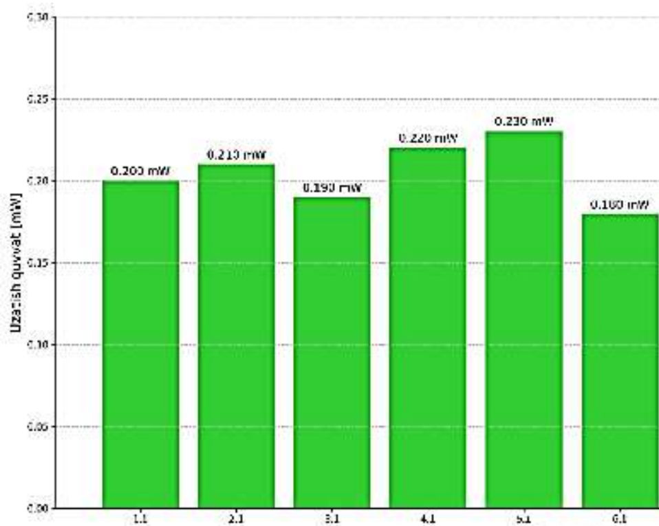
Figure 13: Power consumption of a sensor node during data transmission (transmission)
