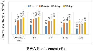
Figure 2: Chart represent compressive strength of concrete containing BWA
