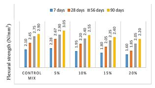
WSA Replacement (%) Figure 5: Chart represent flexural strength of concrete containing WSA
