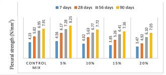
WSA Replacement (%) Figure 3: Chart represent flexural strength of concrete containing WSA
