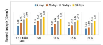
BWA Replacement (%) Figure 6: Chart represent flexural strength of Concrete containing BWA
