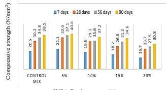
WSA Replacement (%) Figure 1: Chart represent compressive strength of concrete containing WSA
