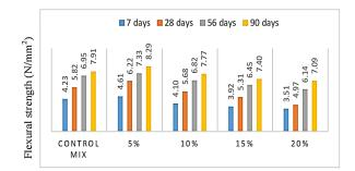
BWA Replacement (%) Figure 4: Chart represent flexural strength of concrete containing BWA
