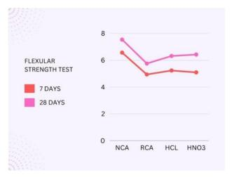
Figure 3: Flexural strength test line diagram
