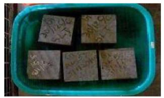
Figure 3: Sample dipped in Diluted 5 % Sodium Sulphate Solution
