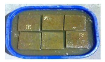
Figure 2: Sample submerged in 3% diluted sodium chloride solution
