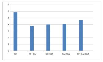
Figure 10: Percentage of Strength drop on Resistance of sulphate
