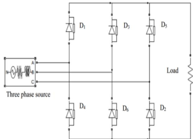
Figure 2: Circuit Diagram of a Three Phase Rectifier Working of a three phase rectifier is described as follows:
