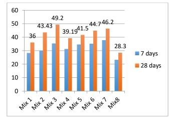
Figure 2: Graph for Compressive Strength
