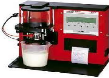
Figure 5. Measuring zeta potential - Mütek SZP-06. (Source: Google Images).
