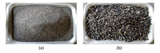
Figure 1: (a) Fine coal bottom ash FCBA; (b) Coarse coal bottom ash CCBA (Hasim et al., 2022)
