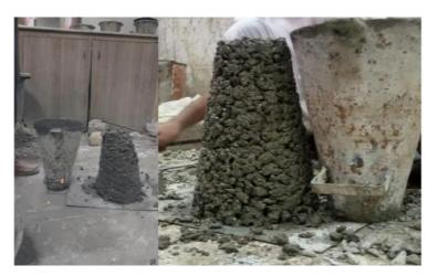
Figure 4: Conducted a slump test (Soomro et al. 2021)
