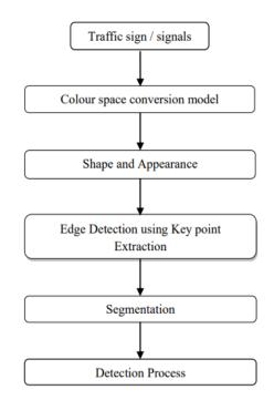
Figure 1: Overview of Image Processing in Traffic Sign Detection.
