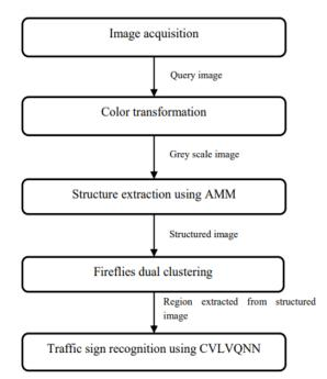
Figure 2: Structure and Flow of the Traffic Sign Detection System
