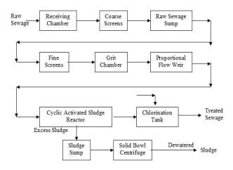
Figure 1: STP Flow Plant
