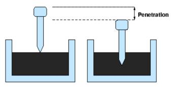
Figure 1: Penetration test setup
