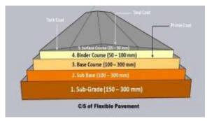
Figure 2: Flexible Pavement
