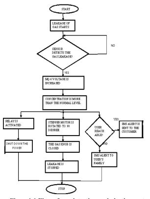
Figure 1.1 Flow of gas detection and alerting system
