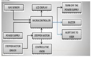
Figure 1: Block diagram for user-interactive gas detection and prevention system.
